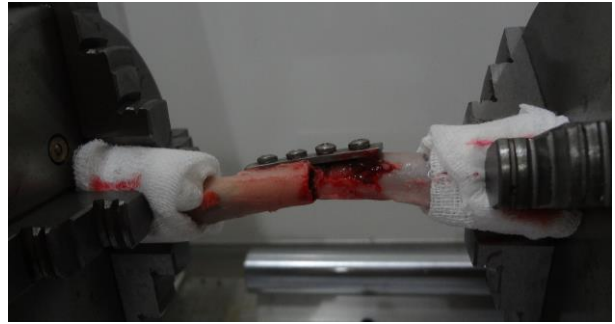
Figure-6. A bone being tested for torsion.
