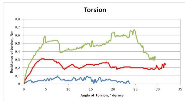
Figure-10. Load torsion angle curves for torsion tests (blue: grooved surface, green: sanded surface, red: smooth surface)
