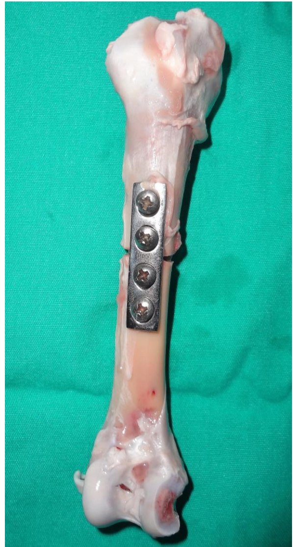
Figure-7. Bones prepared for torsion tests.
