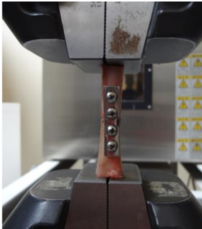
Figure-4. A bone being tested for axial compression.
