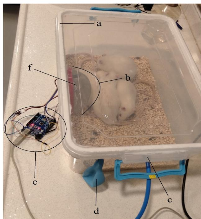
**Figure 1.** Cabinet environment of study group rats (a; Insulating material to prevent air passage, b; Protection of sensors, c; Nitrogen gas inlet, d; Pressure balancing balloon, e; Data transfer module, f; Sensors).
