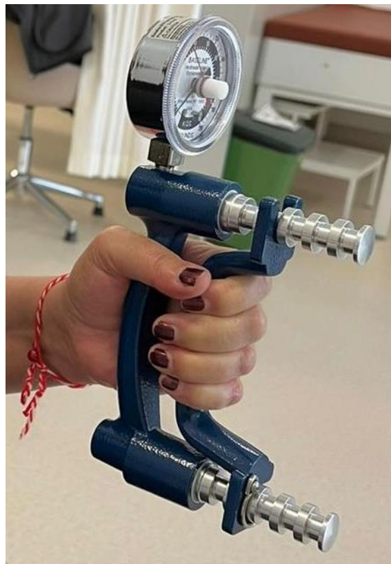
Figure-3. Appearance of the hand dynamometer used in the measurement and measurement of wrist grip strength.
